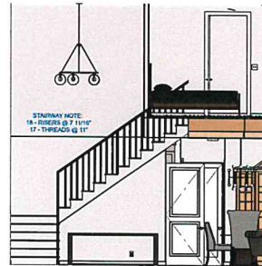
3 STAIRWAY DETAIL SCALE: 1/4"=1'-0"
